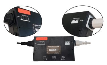
The white cable coming from the Humidifier assembly is for the Low Water Sensor. Plug it into the underside of the Humidistat.
