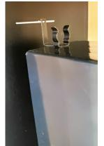
To achieve this height, use either the guide across the top of pages 4 and 5 or place the empty tank on end inside the piano. For a suspended installation, set the tank on the top of the trapwork but mark 3 cm higher than the hole so the tank will clear the trapwork.
