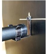
If the Dehumidifier is slightly touching something, loosen the screw and pivot the VDB to gain clearance. Re-tighten the screw when the Dehumidifier is clear of everything.
