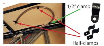
keybed using at least one of the 1/2" clamps and the two half clamps. It can be curled up as shown below. Attach the clamps with the short screws.
