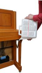
Tip the can so the nozzle points down. Take care not to tip too far when the can is full. When the watering can is empty, but before separating the watering tube from the can, set the can on the floor and let any water remaining in the tube drain back into the can. Pull the nozzle out of the watering tube and replace the tube into the half clamps under the keybed or wherever it was originally.
