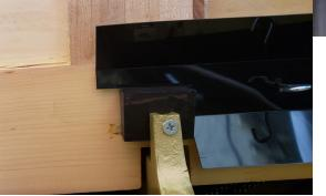
You may need to trim the baffle with scissors to clear plate struts. You may opt to secure the baffle by using the push pins as well. Pushing them through the Velcro© works well.
