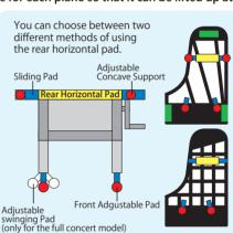
If the wood frames are in a lower position to the underside of the side board and if you do not want the wood frames to bear the load by themselves, attach the concave supports to the rear horizontal pad and support the load with the side board.
